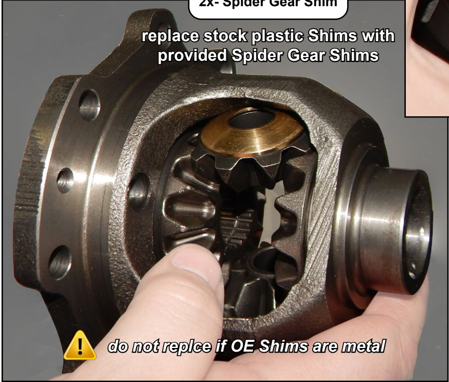
2x- Spider Gear Shim
