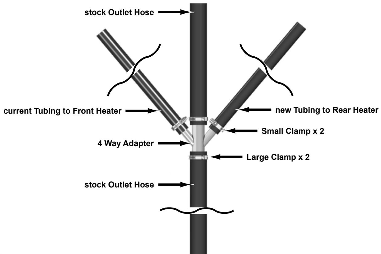
To prevent stock Radiator Hoses from being cut short, use provided Adapters as templates.
