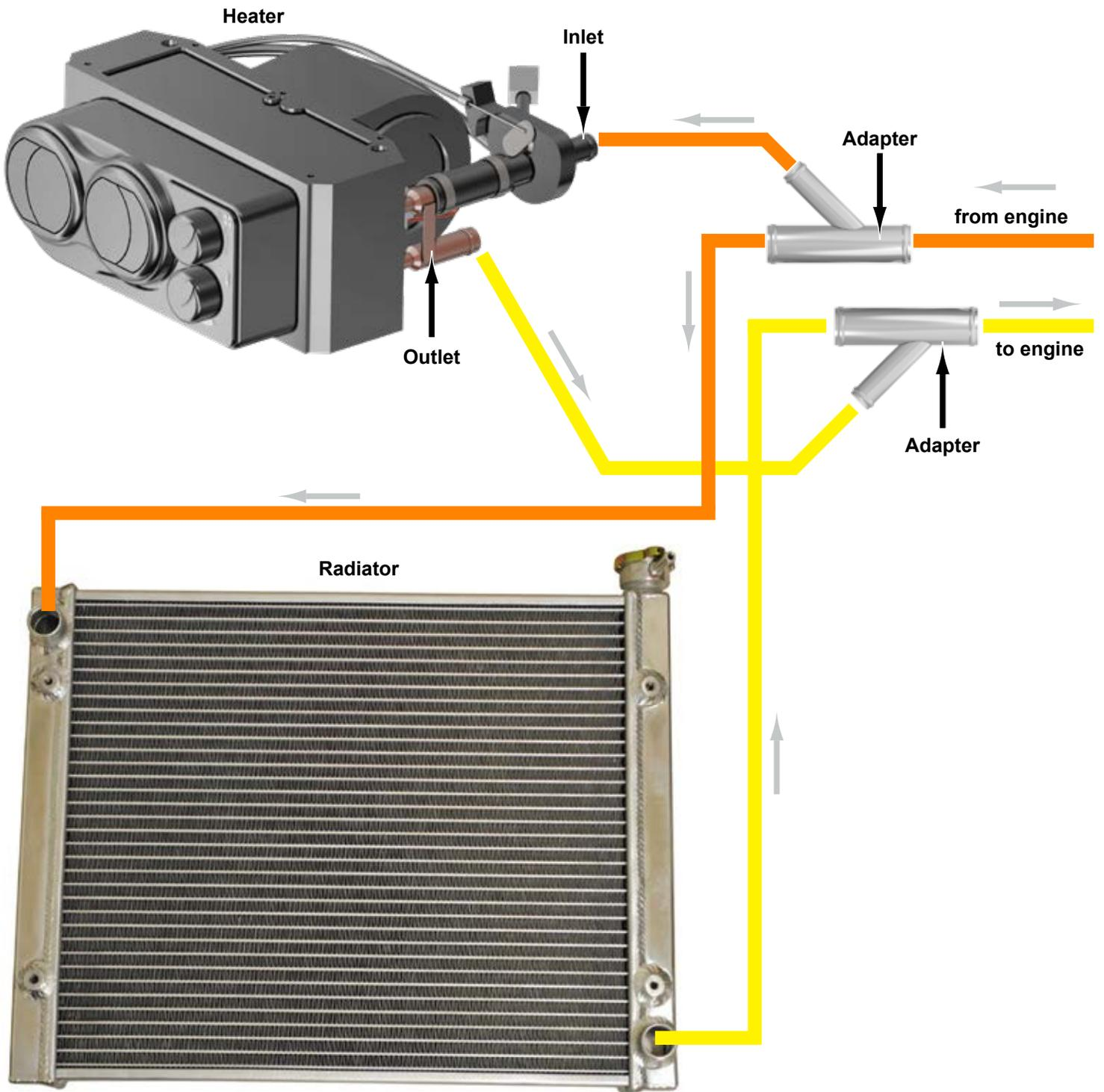
**IF NO FRONT HEATER IS PRESENT, OR NOT BEING INSTALLED AT THIS TIME,
