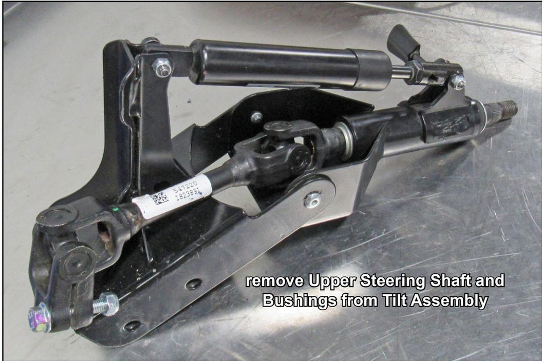
remove Upper Steering Shaft and Bushings from Tilt Assembly
