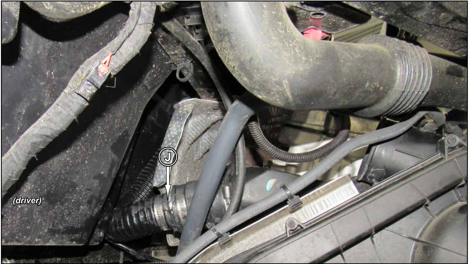
IN-SKL-P-GEN Route Belt Intake Snorkels (J) up and behind Air Box.
